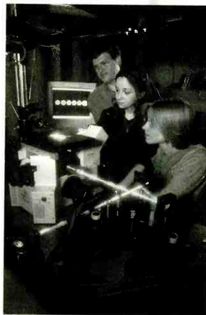
Robert Dickson, Lynn Peyser, and Amy Vinson expose a silver nanocluster sample to green laser light. Responses are shown on the computer monitor behind them. (Photo by Gary Meek)
