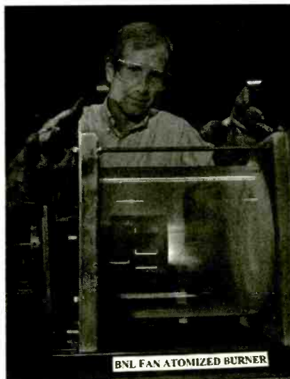
Brookhaven National Laboratory (BNL) researcher Thomas Butcher inspects the flame pattern in the BNL fan-atomized oil burner.
