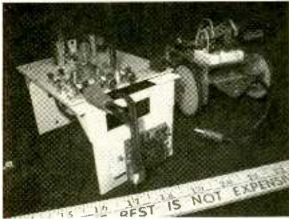
The completed EYEBot frame is ready for mounting on the BOEBot.
