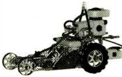
A combination robot/hot rod (another bonus plan available from the CyberK'NEX Web site). A motor is located at the rear of the robotic vehicle; a motor-control pad is located in the "driver's" seat.
