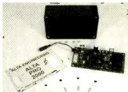
The Alta Pro 2000's PC board is mounted to the lid of the case using screws and spacers. You might need an additional IC socket to raise the ZIF socket to the proper height.
