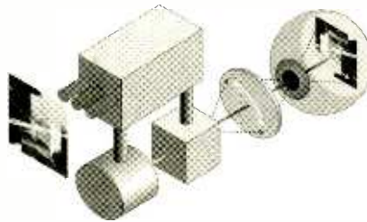
Fig. 1. The Microvision Virtual-Retinal Display consists of four main parts to translate the source image from a computer or camera into an image projected on the eye’s retina: drive electronics, a modulated light source, horizontal and vertical scanners, and viewing optics.
