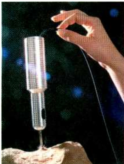
This drill, developed at NASA's Jet Propulsion Laboratory, weighs about a pound but can drill with a jackhammer-like motion through rock as hard as granite or basalt. The broken debris is drawn up through the hollow drill shaft. The resulting hole is little bigger than the drill head.
