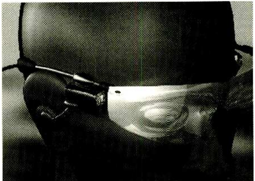
Fig. 2. An artist’s interpretation of a “see-through” head-mounted display using VRD technology.
