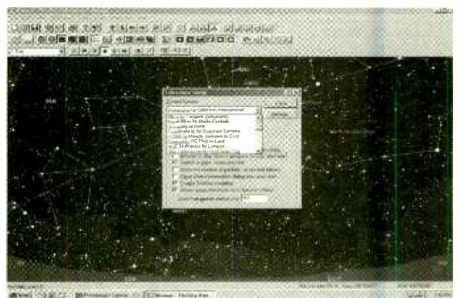
You need to specify the type of GOTO scope or controller that you are using. Initially, as shown here, The Sky did not have an entry for the NexStar5. A patch downloaded from The Software Bisque's Web site fixed that.
