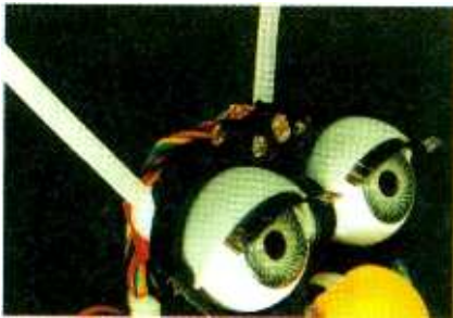
This Furby's head, stripped of its outer covering and fur, reveals the light sensor between the eyes. On either side are infrared transmitter and receiver LEDs. Furbys can automatically communicate with one another via this infrared link.
