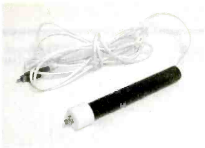
Fig. 9. Each game handle is a length of PVC pipe with a momentary-contact pushbutton mounted on an end cap. Painting the handles an appropriate color gives the GameEnhancer a slick look.
