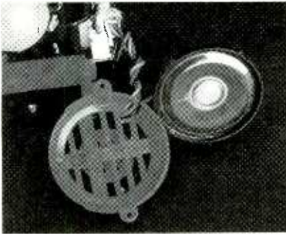
The Furby's 2-inch speaker is capable of very clear sound reproduction.
