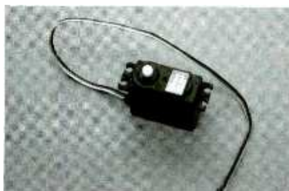
Fig. 1. A typical radio-controlled (R/C) servo motor.
