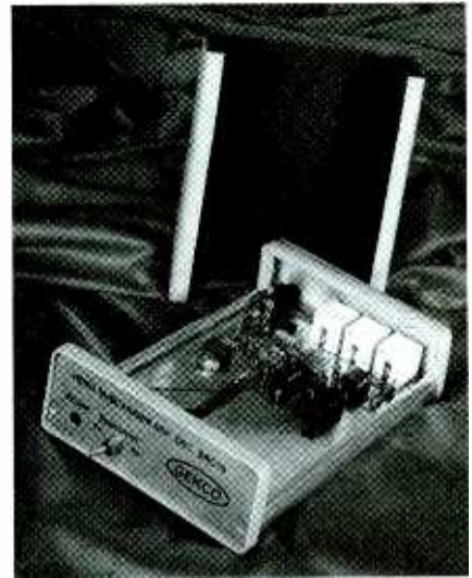
Once the completed Colorburst-Calibration Reference is installed in a case and closed up, it's ready to be a trusty, always-available assistant on your workbench
