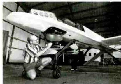
Sandia researcher Bill Hensley checks the Lynx SAR installed on a General Atomics I-GNAT unmanned aerial vehicle. (Photo by Randy Montoya)
