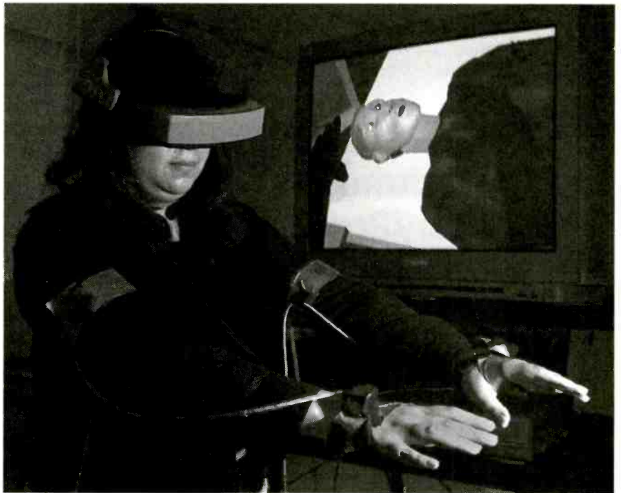
Lydia Tapir of Sandia demonstrates BioSimMER, a virtual reality application that allows rescue personnel to practice responding to a terrorist attack involving the release of a biological agent following a bombing. Through her goggles, she sees the scene shown on the screen behind her where a virtual patient exhibits realistic symptoms from a severe head wound. (Photo by Randy Montoya)
