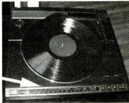
These buttons on the Carrera turntable let you program the tracks to play.
