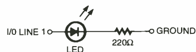
Fig.1. The OOPic can source or sink up to 25 mA per I/O line. This sample circuit drives an LED directly. Transistors or bridges are needed when driving a large relay or a motor.
