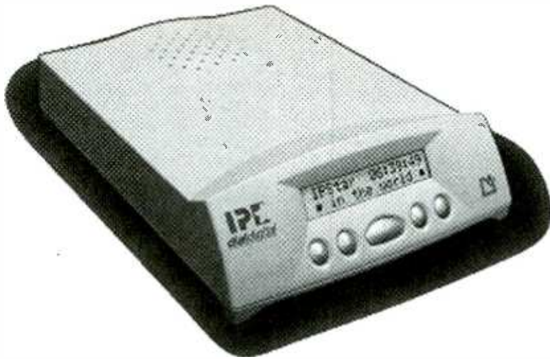
If you'd rather not use a computer for VoIP calls, check out IPStar—a standalone device that handles all aspects of Internet telephony.
