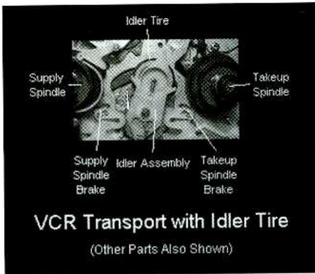
Fig. 2. This VCR mechanism uses an idler tire instead of gears. (Photo courtesy of Brian Siler.)
