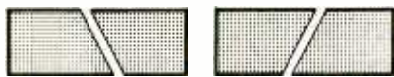
Fig. 3. The azimuth angles of the A and B heads differ—+6 degrees for one and -6 degrees for the other—as illustrated here.
