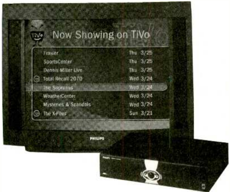
TiVo learns about your preferences and can even pick shows for you to watch. Like ReplayTV, TiVo records video in MPEG-2 format on a hard drive.
