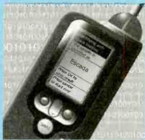
This portable handheld electronic nose from Cyrano Sciences could have applications in many markets.
