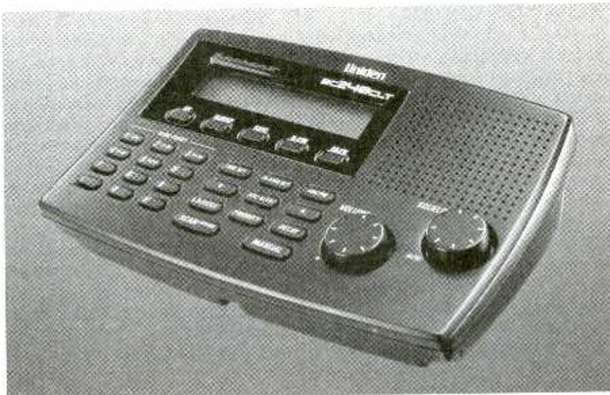
The Uniden BC248CLT takes a novel approach to scanning, by combining a 50-channel scanner with an alarm clock, an emergency weather alert, and an AM/FM radio.
