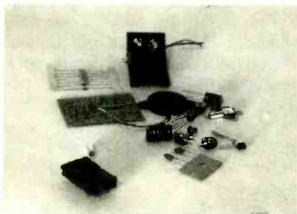
The buzzer used in the project is about 1 1/8 inches in diameter at its circular center and has red (positive) and black (negative) leads to identify their polarities.
