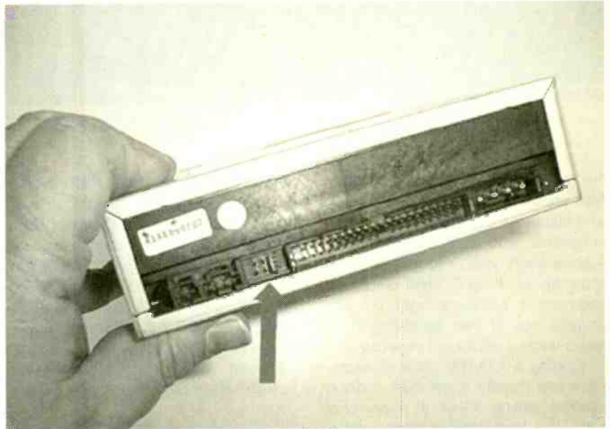
Before installing the CD-RW drive, make certain that the drive jumper is set to the correct Master/Slave status (see text).
