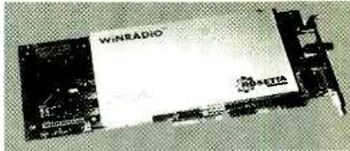
The first generation of computer-controlled receivers, which were prone to RFI generated by the computer itself, were built on ISA cards, and plugged directly into one of the vacant slots on the motherboard of a personal computer.
