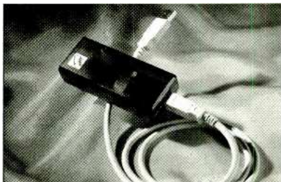
The Leopard Pocket USB modem is about the size of a candy bar, and offers V.90 connectivity in a see-through package.
