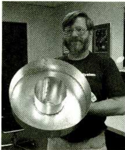
The most common feedhorn for amateur SETI use is a metal pipe, closed off at the end farthest from the dish, forming a shorted cylindrical waveguide. The chief drawback of the cylindrical waveguide feedhorn is its large physical size, which actually blocks a part of the dish surface from the "view" of incoming signals, thereby reducing the effective gain of the parabolic antenna.
