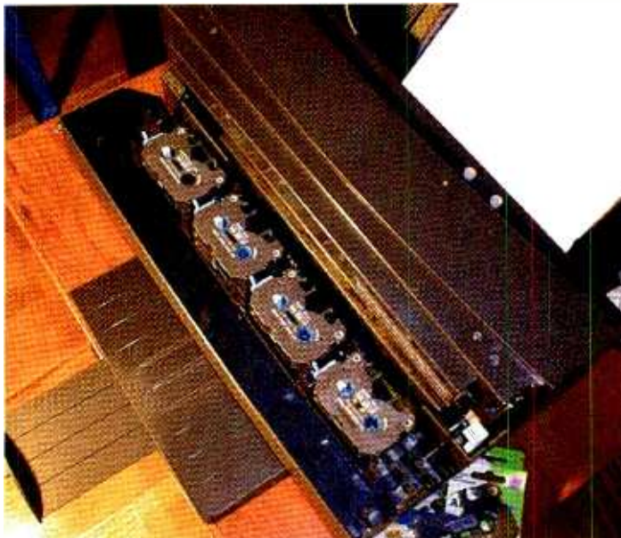
Our foil stamping was done on an Alps MD-5000 printer. Note the cartridges inside—the print head picks up one of these at a time to lay down the individual colors or metallic foils that make up an image.
