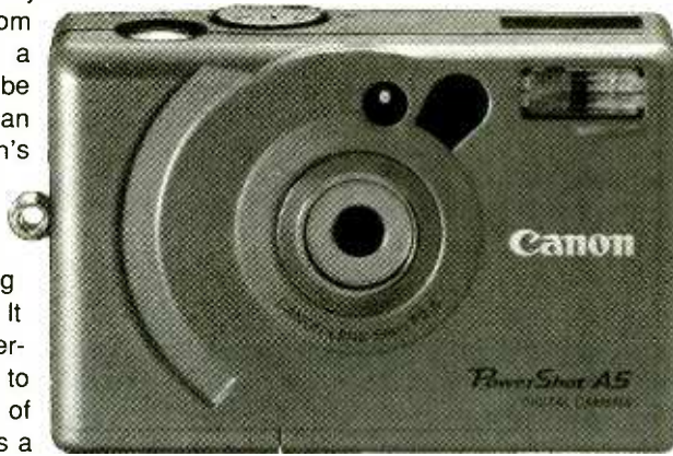
Canon's PowerShot A5 digital camera fits in a shirt pocket and has a maximum resolution of 1024 × 768. It comes with a rechargeable NiMH battery pack.
