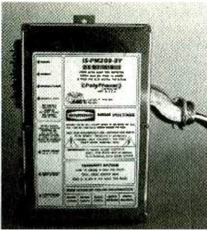
This PolyPhaser AC Line Protector is representative of secondary suppression systems, wherein lightning-based energy is diverted to an outside ground before it enters a building. For best protection, you also should have additional inline, point-of-service surge protectors installed near sensitive equipment.
