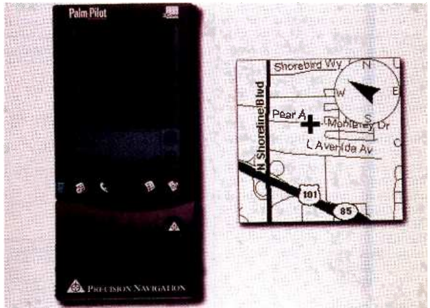
Precision Navigation's Palm Navigator turns a PalmPilot into a compass-aided map navigation system.
