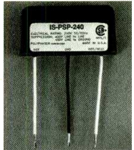
This PolyPhaser device is designed to protect military and other high-end equipment. Designed to provide both MOV- and high-current gas-tube protection internally, the unit is intended to be hardwired and soldered into place within the electronic equipment or appliance it protects.
