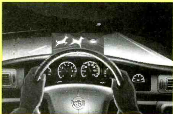
The head-up display projects a virtual image onto the windshield, allowing the driver to keep his eyes on the road.
