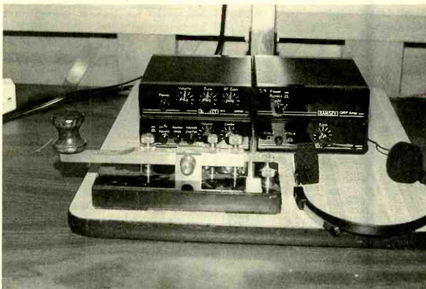
My QRP station consists of four Ramsey kits—a direct-conversion receiver, a transmitter, a power amplifier, an audio filter—and a telegraph key (made by Stillwell in England). The earphones are modern RadioShack $8.95 specials.
