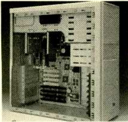
Your computer exposed! Here is a side view with panel removed showing the installed (ATX) motherboard.
