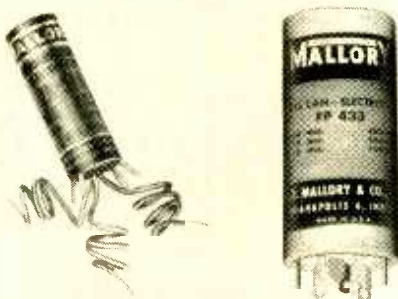
Two styles of multi-section electrolytics. You'll be replacing such caps with equivalent individual units.
