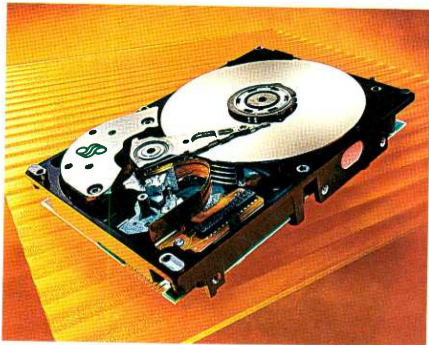
Pictured here is Seagate's Cheetah 9LP hard drive, which has the fastest average seek time of any Winchester-type disc drive, as low as 5.2 msec during read operations. The drive also delivers top performance with sustained data transfer rates reaching over 20 Mbps.
