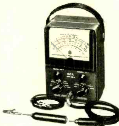
An RCA VoltOhmyst Junior like this one (or its "Senior" big brother), if in good shape, will serve well as your basic multimeter.
