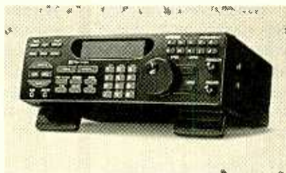
The BC-9000XLT provides frequency coverage from 25-1300 MHz, NFM, WFM, and AM. The frequencies can be stored in 500 memory channels, which are set up in 20 banks of 25 channels each.
