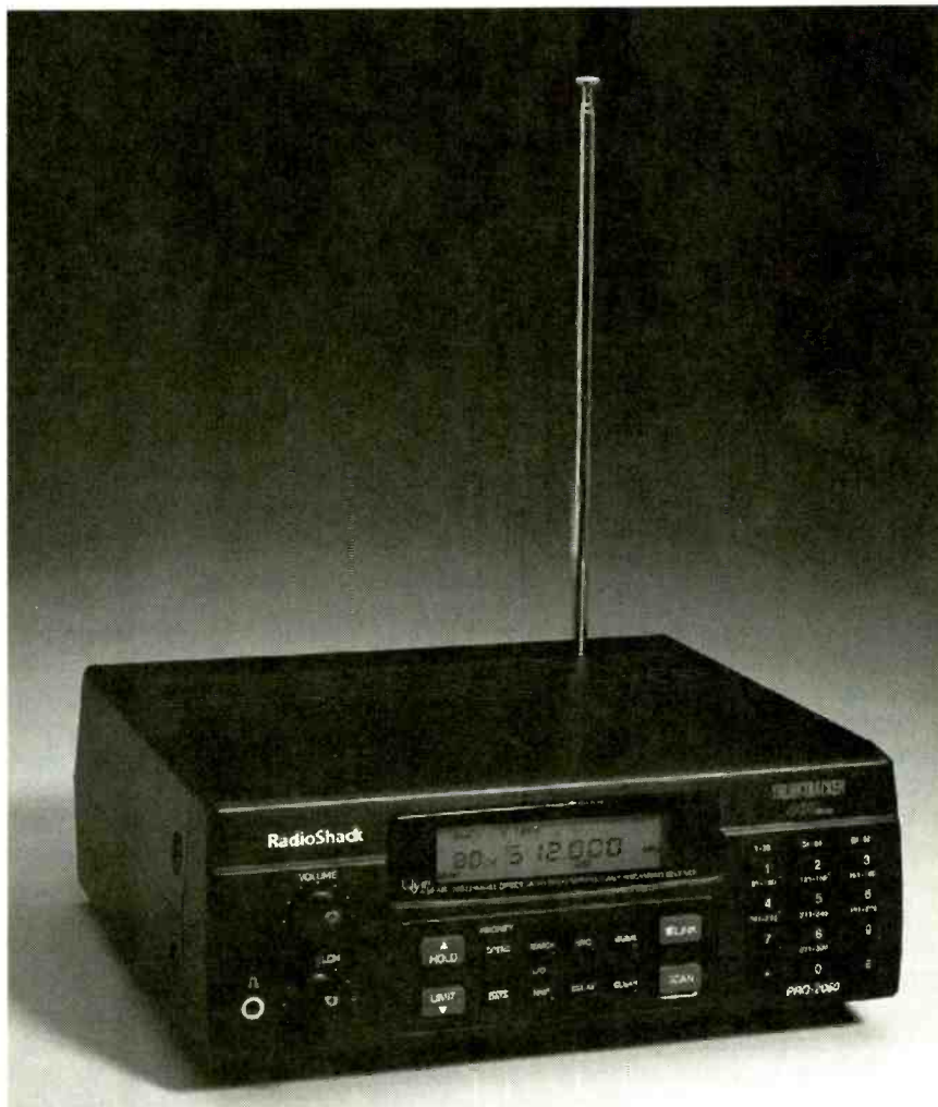
In its trunking mode, the PRO-2050, a desk-top TrunkTracker-unit from RadioShack will easily follow a conversation as it quickly switches from one frequency to another within the group of channels used by a trunked system licensee.
