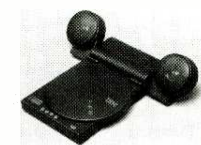
This portable CD-ROM drive from IBM has a fast PC-card interface to provide any notebook computer having a compatible slot with a CD-ROM drive, sound, and speakers.
