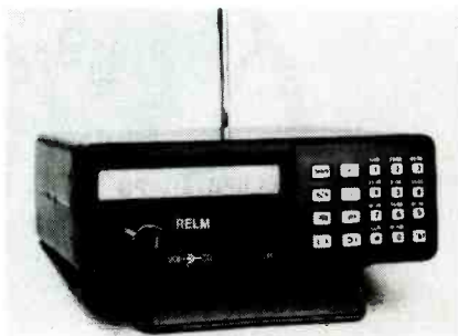
The Relm MS-180, which holds 100 memory channels, covers the 800-MHz band.
