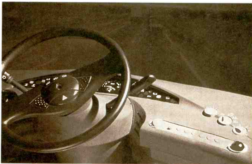
Shown here is the TRACS cockpit used for simulated training of professional truck drivers.
