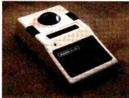
ITAC Systems' Personal Mouse-Trak features a wrist pad and trackball, along with three mouse buttons.
