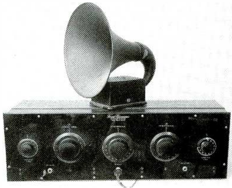
Buttoned up, back in its cabinet, and ready for action, the NR-5 stands by with a "Dictogrand" horn (one of my favorites).
