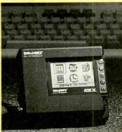
The compact REX docking station is used when no PCMCIA slot is available.
