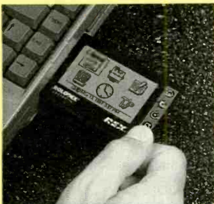
If your laptop or desktop PC has a PCMCIA slot, you can simply slide REX in to download data.
