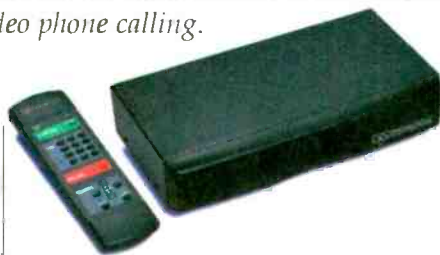
The C-Phone Home is about the size and shape of a cable TV converter box, and hooks up to the TV just like a VCR. Your television set is used to present the audio and video of the person being called.
