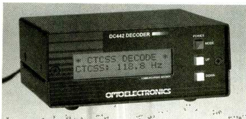
The Optoelectronics DC442 Decoder can be used with any scanner or receiver. It automatically and instantly provides a readout of DTMF, CTCSS, and DCS data.
