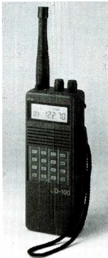
The JD-100 by JAL Data is a specialized aircraft communications scanner.
