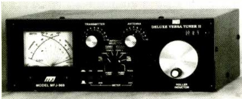
MFJ Deluxe Versa Tuner II is designed for rigs rated at 300 watts and under.
