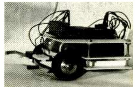
Fig. 1. This simple robot roams aimlessly, but if it hits a wall or other obstacle, its single behavior causes it to back up and turn in another direction.
