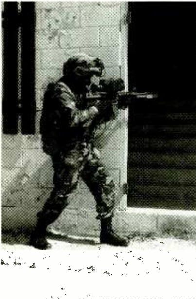
This soldier is equipped with the Land Warrior System. A computer, radios, GPS receiver, antennas, and batteries are carried in a compact backpack.
