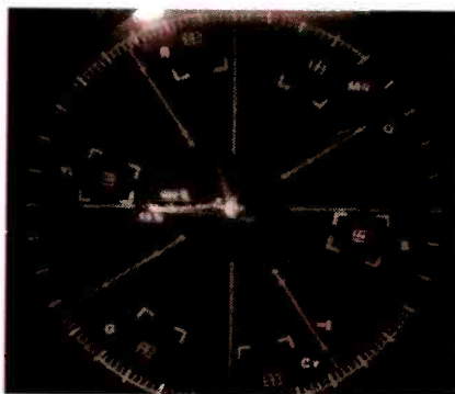
Fig. 1. As this vectorscope photo shows, the ES6000's phase is right on target while its chroma—at the rim of the scope, above the crosshairs—is slightly oversaturated.
