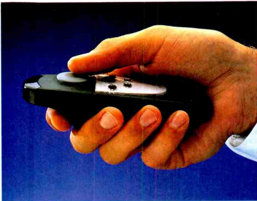
Interlink's RemotePoint Plus is a handheld wireless infrared (IR) mouse. In addition to primary (left) and secondary mouse buttons, it has four extra buttons that can be assigned to as many as 15 functions to access presentation tools, start games, mute sound, launch a Web browser, and so on.
