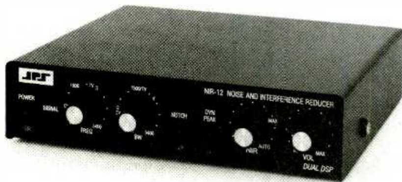
A popular DSP receiver enhancement device is the JPS NIR-12 Dual DSP Noise/Interference Reduction Unit. The NIR-12 provides "spectral subtraction" noise reduction in addition to dynamic peaking. The spectral subtraction mode is effective in reducing impulse noise.
