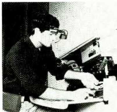
The Mobile Assistant allows for complete "hands-off" operation as this technician follows a visual test/repair procedure on complicated military equipment.
