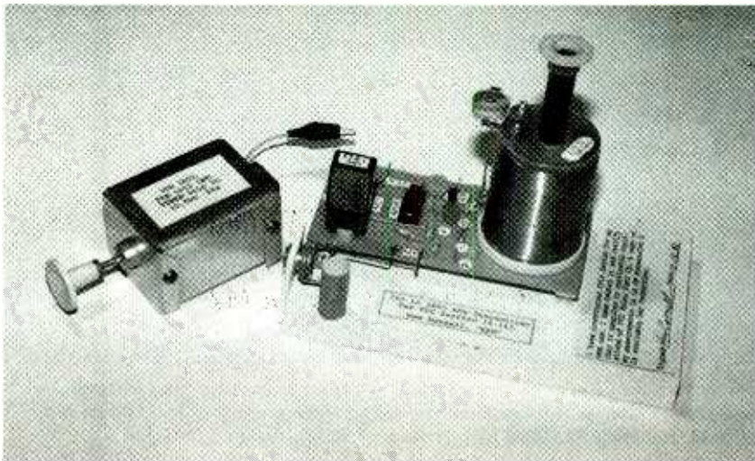
Shown here is a crystal-controlled MedFERS transmitter, circa 1975. It uses an enameled wire tank coil and is ferrite-rod tuned. You can substitute a slug-tuned VFO coil for the crystal.
