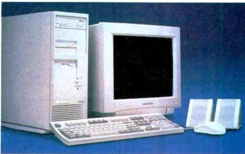
My dual-processor Pentium Pro 200 is more than twice as fast as a Pentium 200, but only with software that can take advantage of the two processors.
