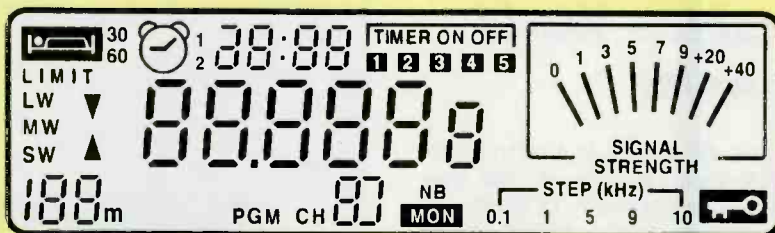
The front-panel LCD provides a very readable display of receiver functions, and includes a liquid-crystal S meter.
