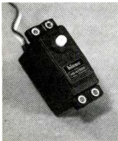
Fig. 3. Here's one of the Hitec HS-425BB servos used in the author's prototype.
