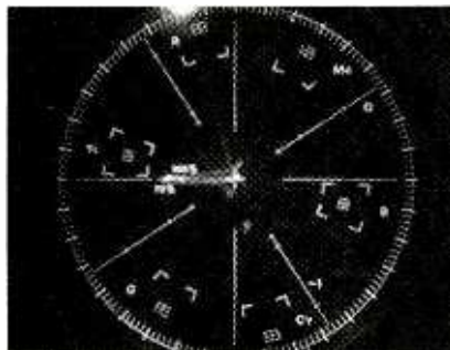
Fig. 1. This vectorscope photograph shows phase to be right on the mark, but chroma (red) to be a little oversaturated.
