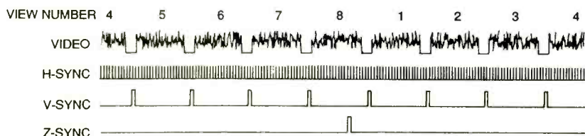
Fig. 5. Here are the drive signals for an eight-view, non-interlaced autostereo image. The entire cycle repeats at 60 Hz.
