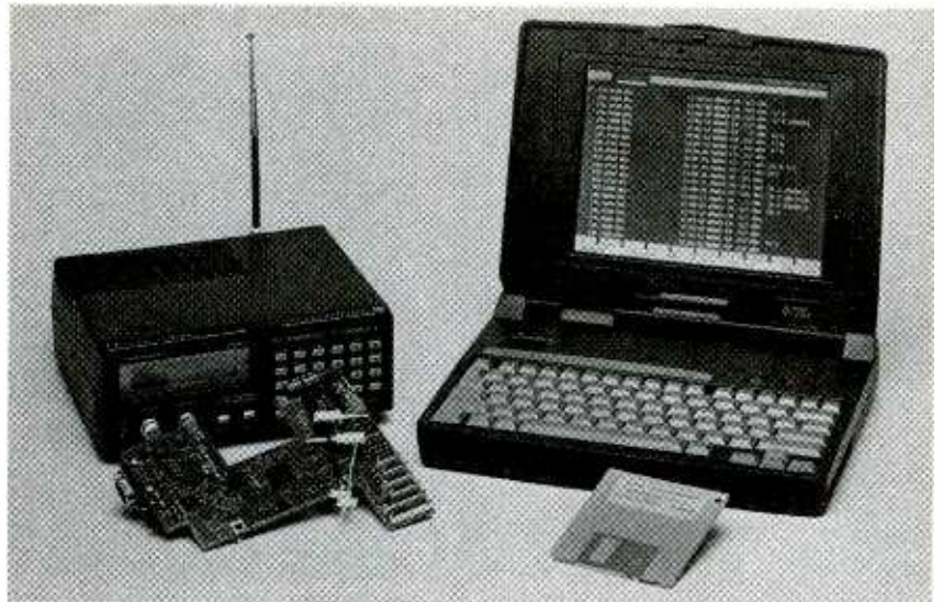
A Radio Shack Pro-2005 scanner equipped with an Optoelectronics OptoScan 456 computer-controlled interface, a PC, and the appropriate software, all form a complete computer-aided VHF/UHF scanning system.
