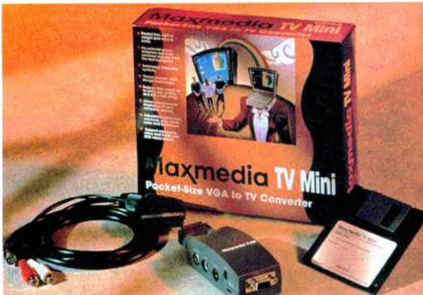
The Maxmedia TV Mini converts the VGA output from a PC into an NTSC or PAL video signal.
