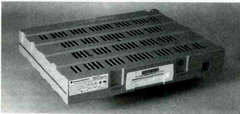
The VideoCipher module: Most consumer satellite receivers are designed to take advantage of it.
