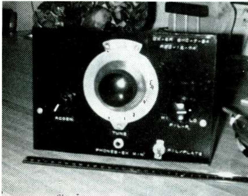
Bob Davey's recreation of "The 2-Tube Short Wave DX-ER" from the July 1934 issue of Short Wave Craft .
