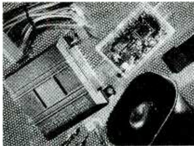
To combat thieves simply "hot-wiring" a car, new theft-deterrent systems, like the one shown in this photograph, will activate if the car is started without the proper key being inserted in the ignition.
