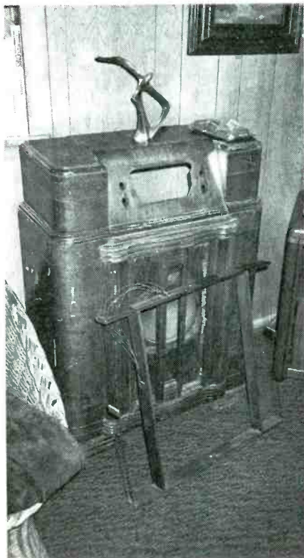
This is the set before restoration. The cabinet has been thoroughly bashed, scratched and scarred. Fortunately, all the pieces were there, and, wonder of wonders, the speaker did not need re-coning. The chassis has been removed for rust removal.
