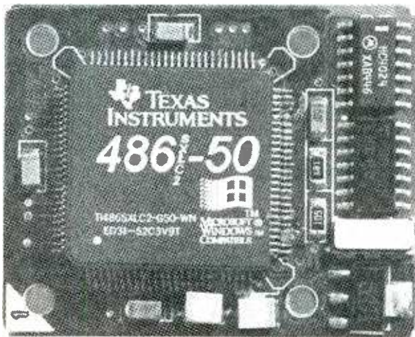
The Make-it 486 will upgrade a 386 computer to a 486 with a built-in 8K cache and a doubled clock speed.
