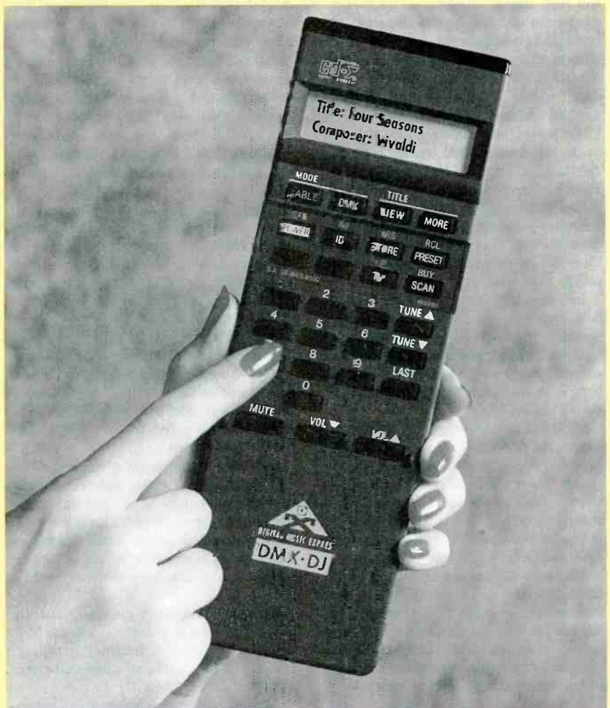
The DMX/DJ remote control allows subscribers to call up the song title, artist, composer, album title, record label, and catalog number of the song they are currently listening to.
