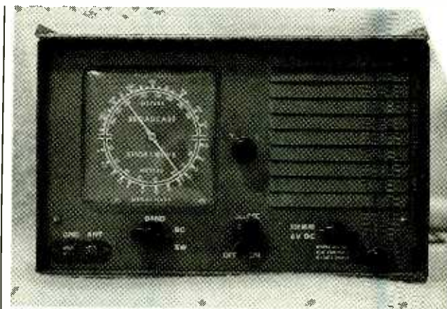
A close-up of 6000-BAC's front panel shows its Spartan layout. The 6/115-volt power switch is under the speaker.
