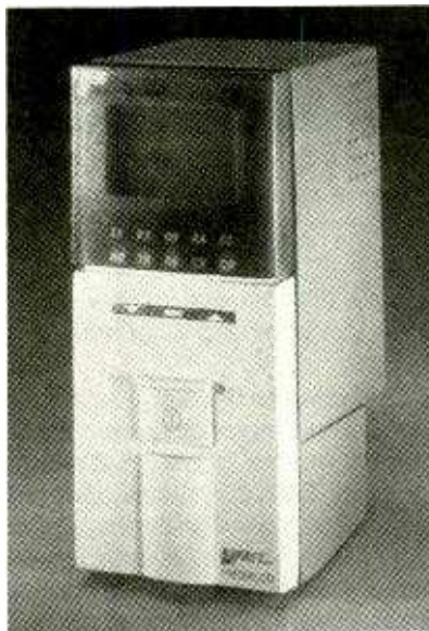
Shown here is a Practical Peripherals 28,800 bps PM288LCD stand-alone modem, which makes use of the fastest speed available over conventional telephone lines.
