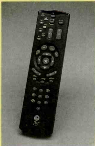
The CB1500's remote control allows the user to navigate through interactive on-screen television listings, activate one-touch recording, and control a TV, VCR, and cable box.
