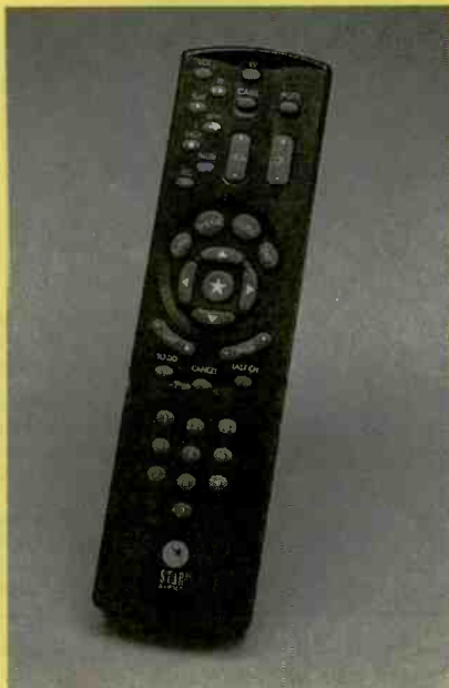
The CB1500's remote control allows the user to navigate through interactive on-screen television listings, activate one-touch recording, and control a TV, VCR, and cable box.
