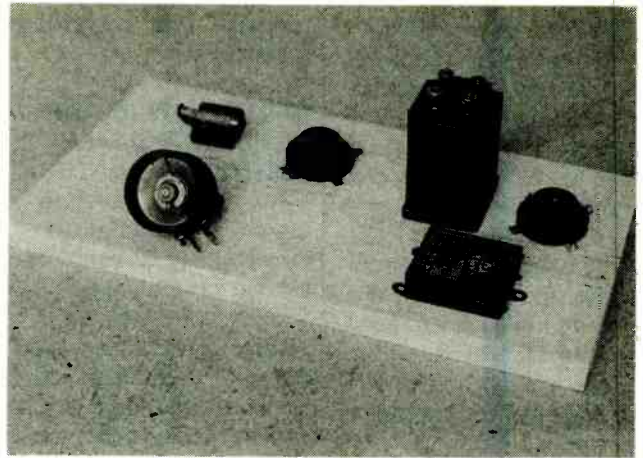
The basic parts were placed on a "breadboard" to check the layout. The board has been ripped down to a 7-inch width (10 inches had been specified) for a more compact parts arrangement.
