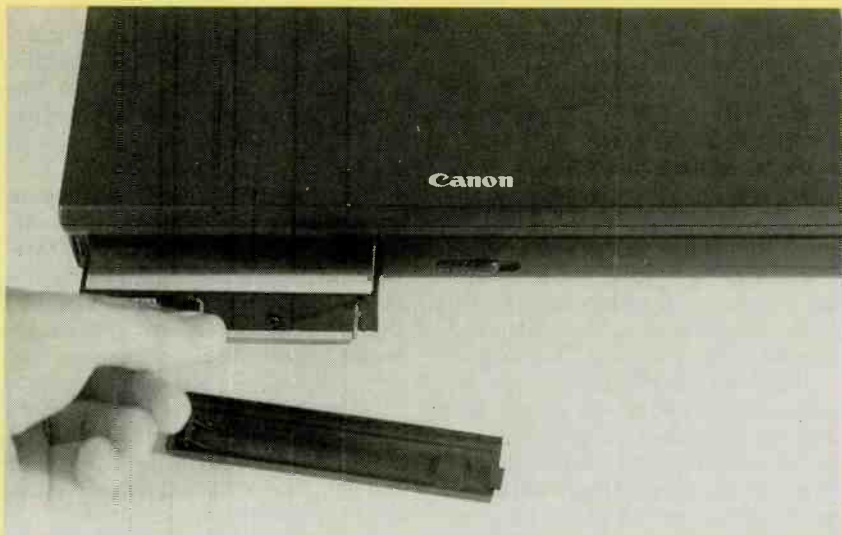
It's easy to upgrade the Innova Book's hard drive. The removable unit can be pulled out and replaced in a snap!
