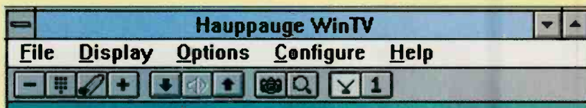
The toolbar provides quick access to the most commonly used functions including channel changing, volume, and freeze-frame.
