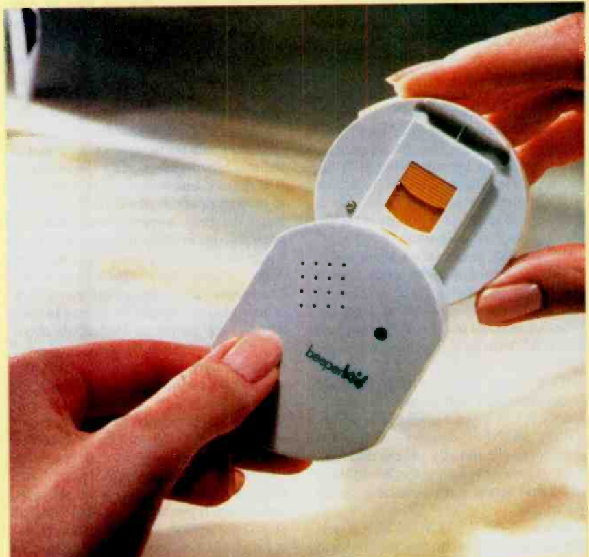
The BeeperKid receiver (front) and transmitter (rear) slide together for easy storage and recharging when not in use. Note the "safety pin" fastener on the back of the receiver, which prevents toddlers from removing the transmitter.
