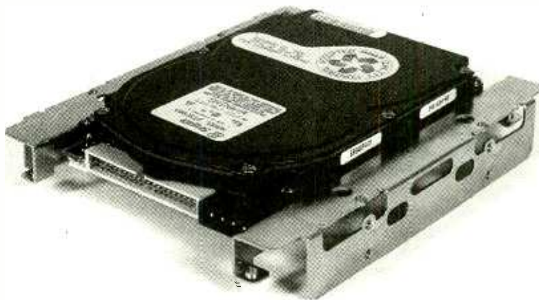
A mounting kit adapts the hard drive to fit in a 5¼-inch drive bay.
