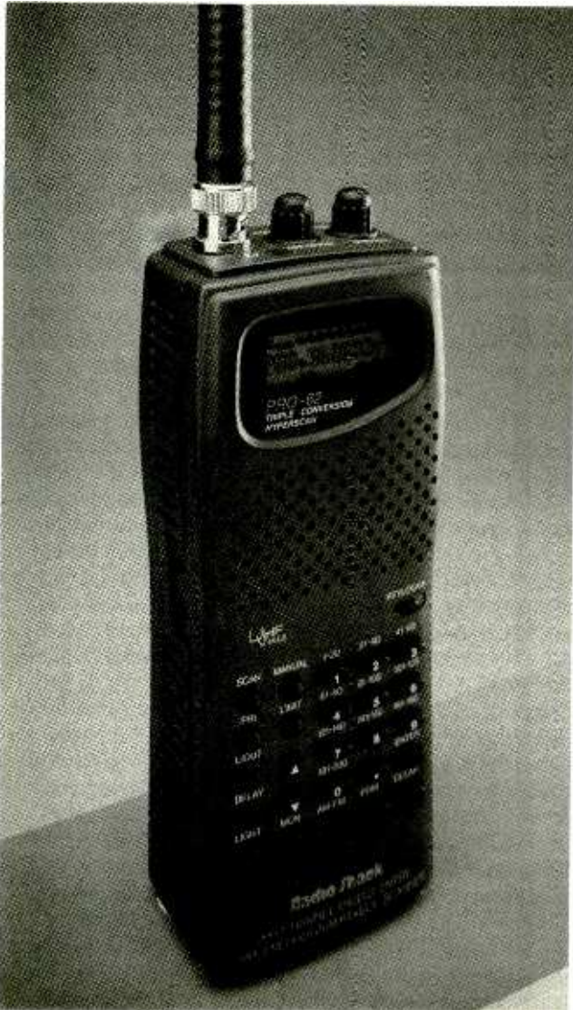
Radio Shack's PRO-62 handheld scanner offers 200 memory channels and covers a wide range of frequencies.
