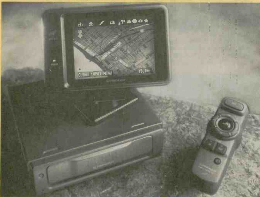
Pioneer's GPS-X77 uses a proprietary map database. The vehicle location is indicated on the moving-map display, and a synthesized voice calls out route-guidance instructions.
