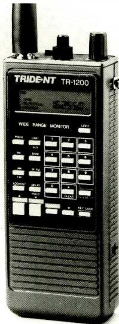
The handheld Trident TR-1200 offers a very wide tuning range and 1000 memory channels.
