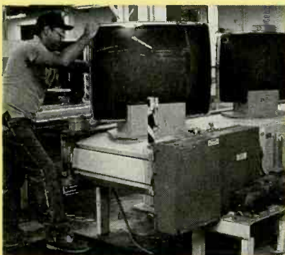
The 40-inch cathode-ray tube, shown being assembled in Mitsubishi's Braselton, GA, plant, is 31% larger in screen area than the 35-inch CRT pictured next to it.
